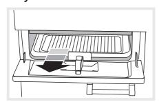
Remove the pan from the bottom of the grill compartment. A cooling fan will start to run as soon as the grill is turned on. The fan will continue to run while the grill (or oven) is on and for about 10min after it is turned off. Never turn off the power supply to the cooker before the cooling fan stops.
